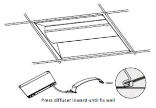
Step7. Press Diffuser (D) inward and make sure fix well. Turn power on. This retrofit kit is on. The installation is finished.
