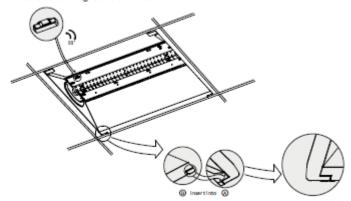
Step6. Install LED panel (B) in between troffer, making sure the tabs at each corner of the LED panel slide into the respective slots on the side panel. Install closing panel (C) in between troffer. Fixate panels and establish ground by turning fastener 90 degrees.
