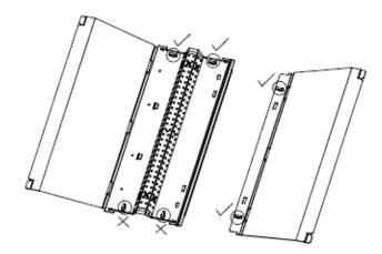
Step3. Fix the supplied fasteners (6 pcs in all) to LED panel (B) and closing panel (C) separately and pay attention to the directions.
