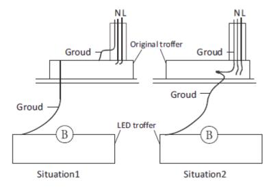
Situation1: Screw grounding cable from LED panel (B) to original troffer if host fixture ground connection is made through host fixture.
