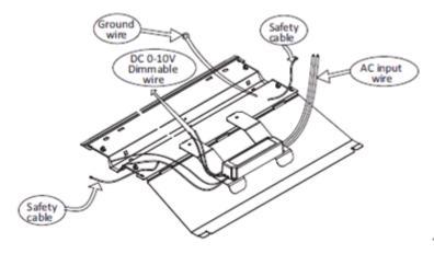
Step5. Connect LED panel (B)'s DC 0-10V dimmable wire, ground wire and AC input wire well. Drill two 4.2mm dim holes in the original bottom troffer by tools. Fixate the safety cable to the bottom troffer by screw.
