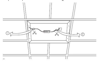
Step2. Remove all the parts such as lamp holder, starter etc. Cut off power wire as shown in ①. If the distance between ballast and ceiling surface is lesser than 3 inch, cut wire ② and remove ballast.
