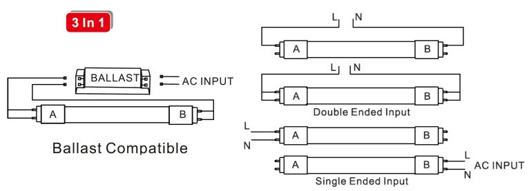
Input voltage: 120-277Vac 50/60Hz
