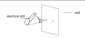
Step 1.Mark the position of the fixing holes with foold lightbracket, then drill the fixing holes.
