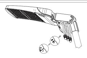
3.Assembling the lamp body of the holder with the bracket, and lock the bracket fixing screws Connect the wires according to the schematic diagram and also make waterproof treatment
