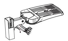
Step 2.Use tools to fix the lamp on square lamp pole, connect the wires correctly and make waterproof measures well, close the junction box and finish installation.
