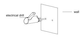
Step 1. Mark the position of the fixing holes with foold lightbracket, then drill the fixing holes.
