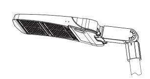
4. Finally, lock the bracket wiring cover plate to complete the installation
