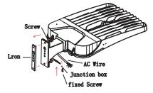
Step 1.Use tools to take screw apart and put installed iron bar away, remove fixed screw and open junction box, then pass the AC wire through it.
