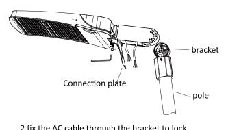
2.fix the AC cable through the bracket to lock it on the lamp body;
