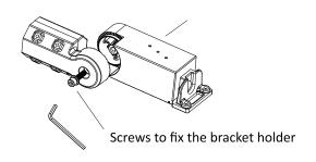
1.Use a wrench to loosen the fixing screws on the bracket, remove the bracket, and then use a screwdriver to remove the bracket wiring cover screws
